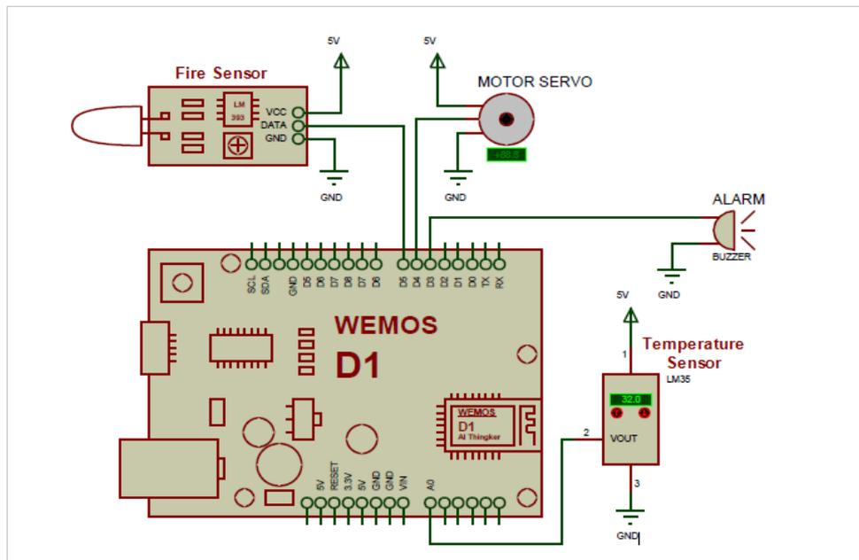
Figure 1: A prototype circuit for an early fire detection device.
